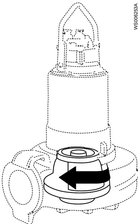
The correct direction of impeller rotation is clockwise when you look at the pump from above.
