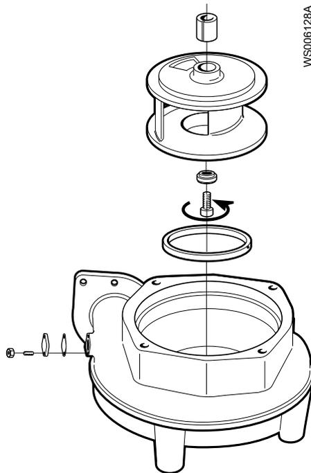
Figure 13: C-Impeller
