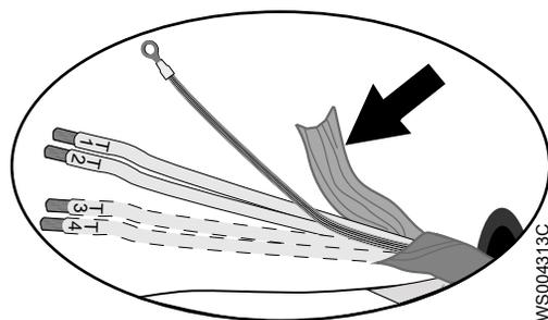
Figure 10: Copper foil on control element.
