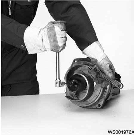
3. Remove the impeller.
