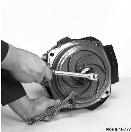
3. Refit the impeller screw.
