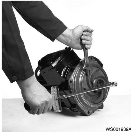
Check that the impeller can rotate freely.
