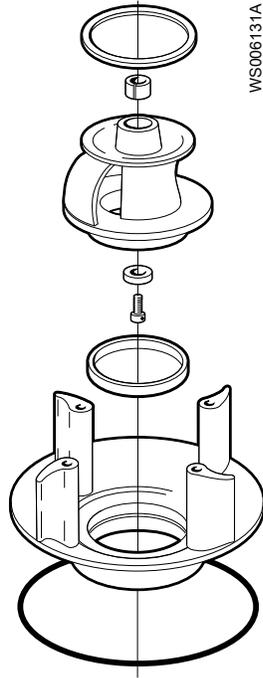
Figure 15: L-impeller
