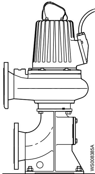
Figure 4: T-installation
