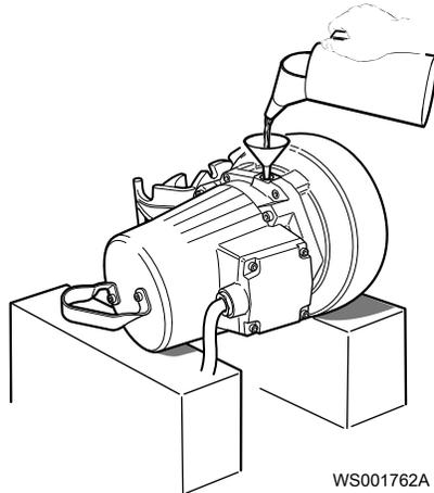
4. Refit the oil plug and tighten.
