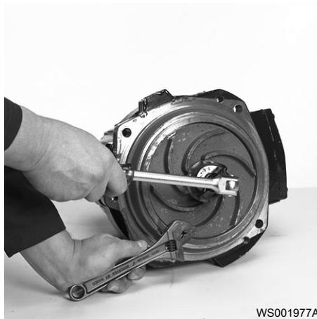
3. Refit the impeller screw.
