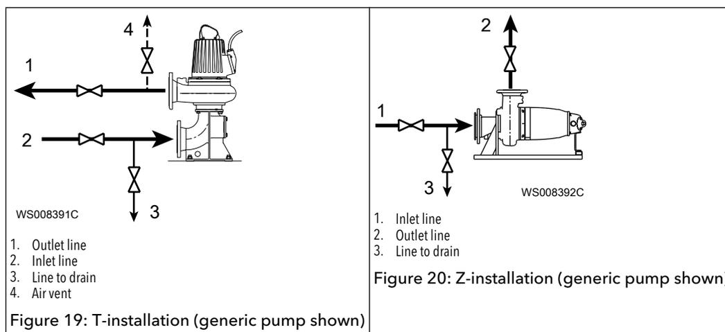
2. Drain the pump by opening the valve on the drain line.
