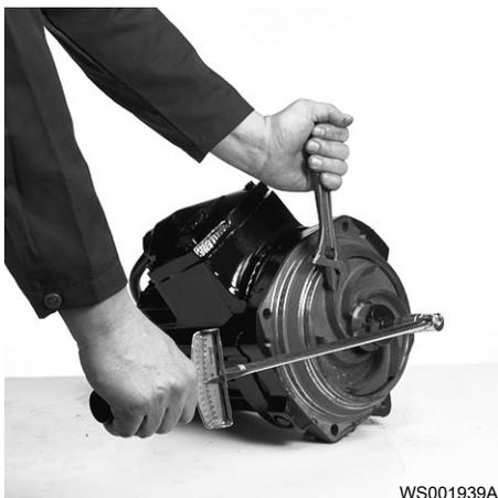
Check that the impeller can rotate freely.
