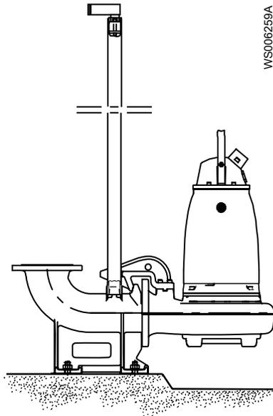
Figure 2: P-installation
