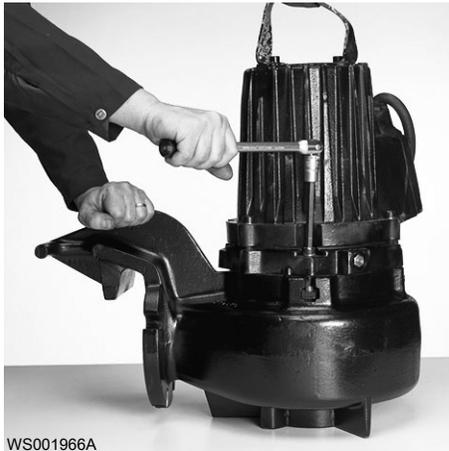
2. Remove the impeller screw.
